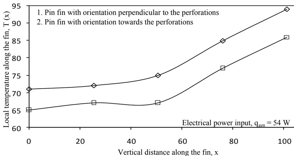
Fig. 4 Temperature profiles of a pin fin with change in orientation
