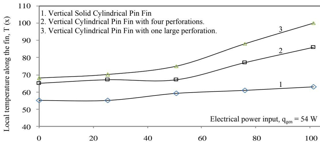
Fig. 2 Temperature profiles along the fin with and without perforations
