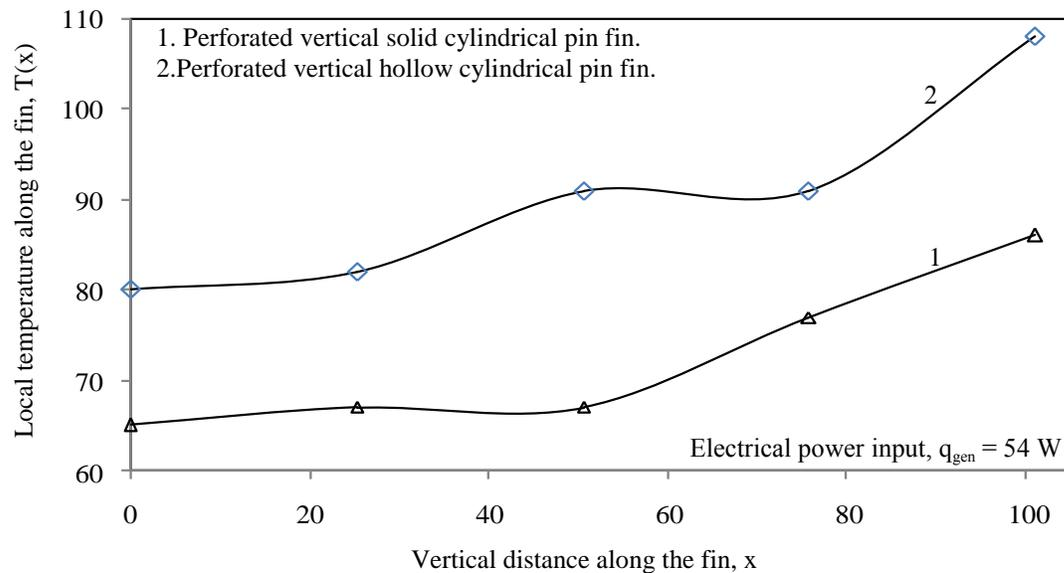
Fig. 3 Temperature profiles for solid and hollow perforated fins
