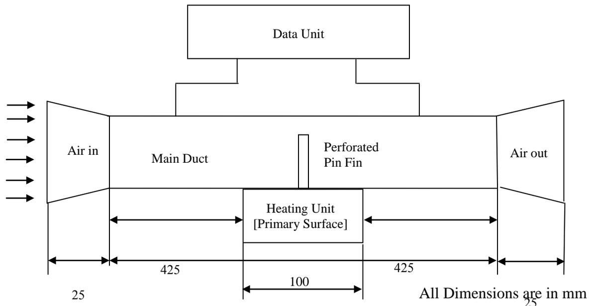
Fig. 1 Schematic of the experimental set up used for the study.
