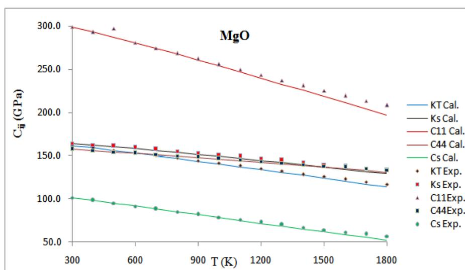
Fig. 1 Temperature dependence of elastic constants for MgO
