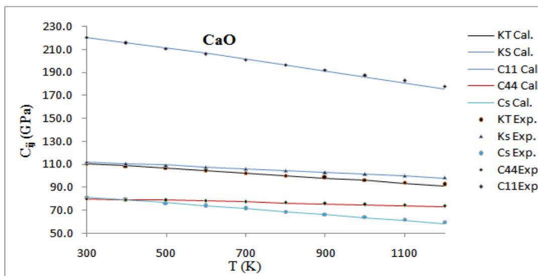
**Fig. 2** Temperature dependence of elastic constants for CaO
