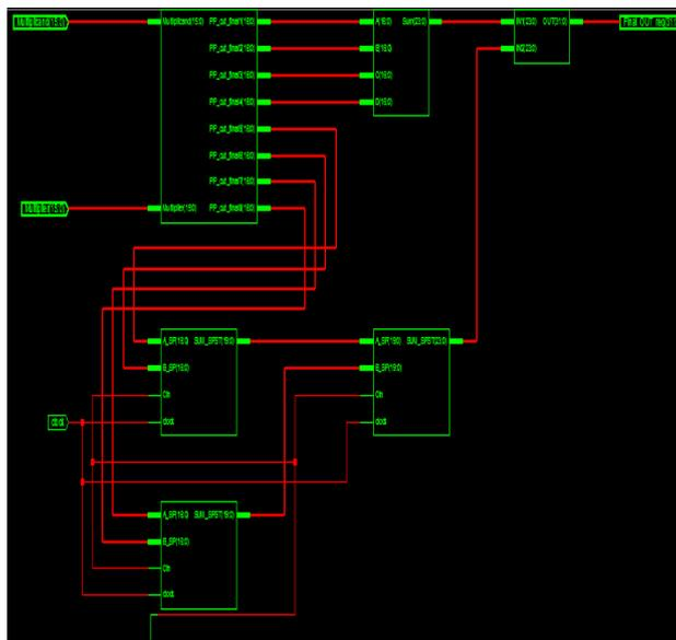
**Fig 4.2: Synthesis results of multiplier**
