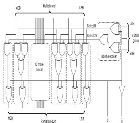
Fig 3.1.1: Block Diagram of Partial Product
