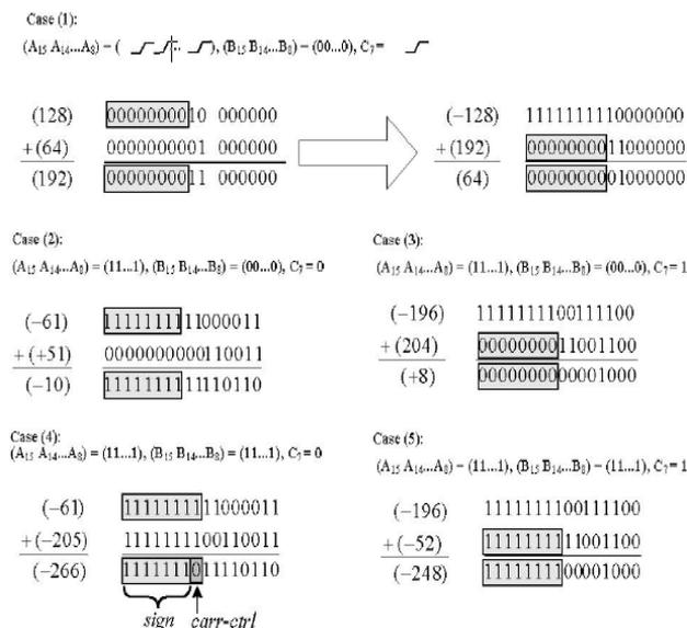
Fig 3.2.1: Spurious transition cases in multimedia/ DSP processing
