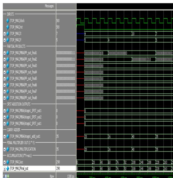
Fig 4.1: Simulation results of Booth encoder
