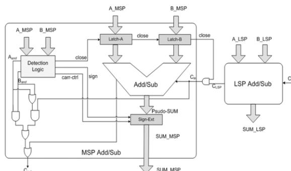
Fig 3.2.2: Low power adder/ Subtractor adopting the SPST.
