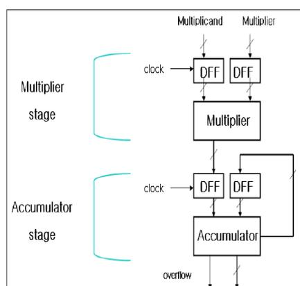
Fig 2.1: Simple Multiplier and Accumulator Architecture
