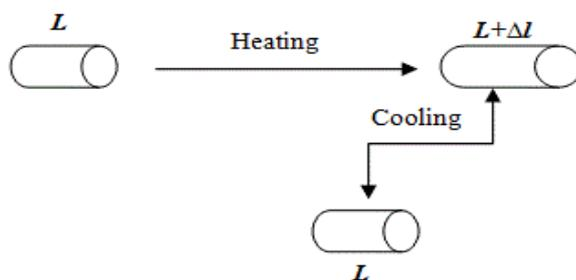
Figure 3. dilatometry procedure
