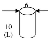
Figure 2 Sample dimensions(mm)
