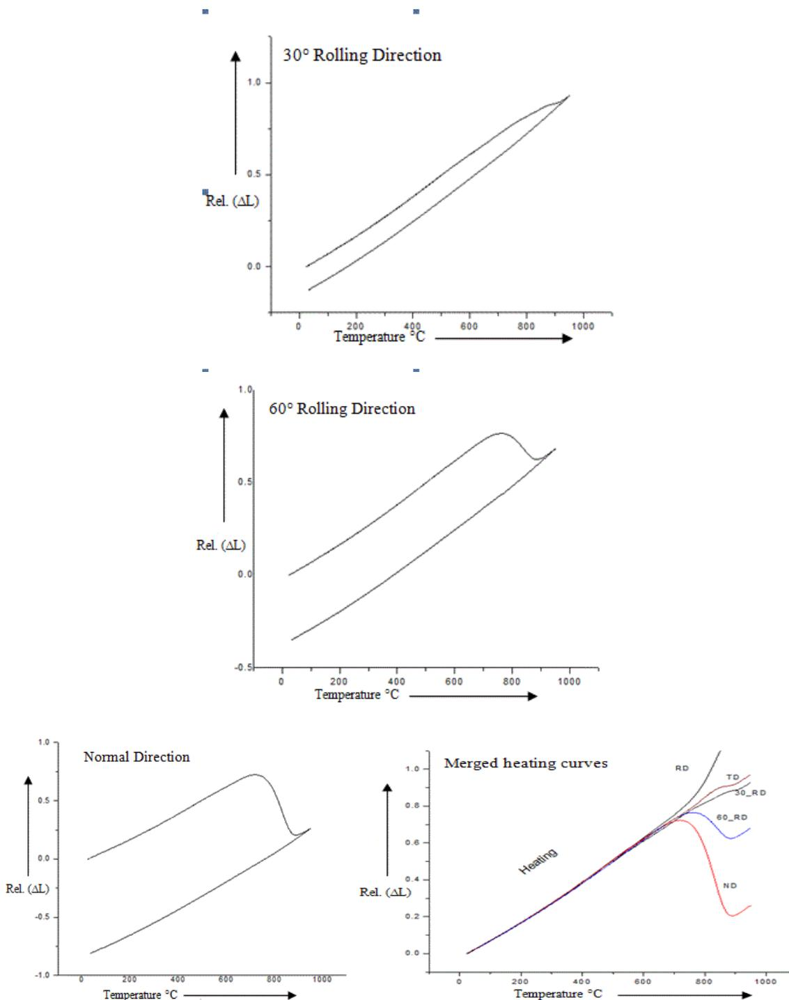
Figure 4. Dilatometry curves.
