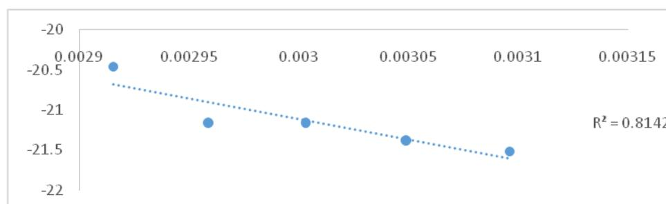
**Figure 3: Plot of ln D versus Temperature Inverse**
