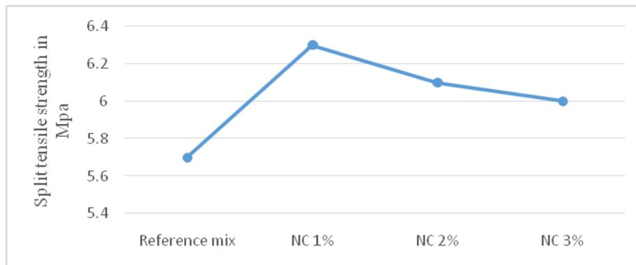
Fig -2: Variation of 28 days split tensile strength of HSC with Nano CaCO<sub>3</sub>.
