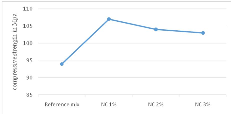
Fig -1: Variation of 28 days compressive strength of HSC with Nano CaCO<sub>3</sub>.
