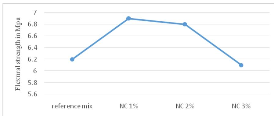
Fig -3: Variation of 28 days Flexural strength of HSC with Nano CaCO<sub>3</sub>.
