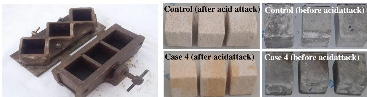
**Fig. (2) Specimen's Molds and Specimens Cement Mortar with and without Microorganisms, Before and After Acid Attack**
