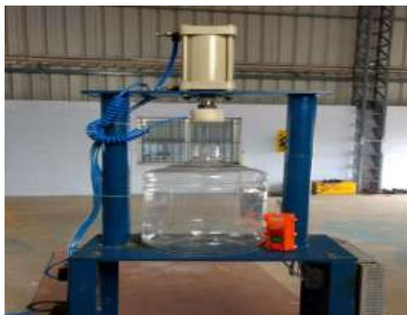
Fig .2 Leak Testing Machine
