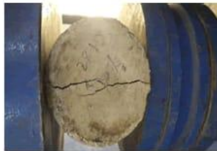
Figure 5: Failure of specimen along with wood ash.
