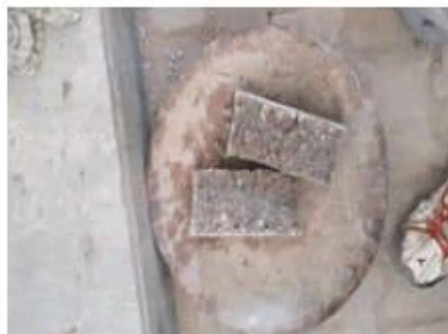
Figure 4: Failure of control specimen.
