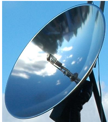
Photo 4. Parabolic Dish collector
