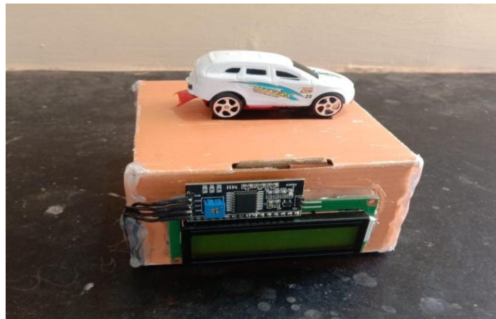
Figure 3: Parking Slot With IR sensor and LCD Display
