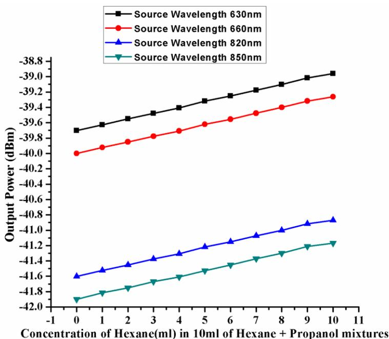
Fig.4: Relation between Concentration of Hexane(ml) in 10ml of Hexane + Propanol mixtures Vs Output Power(dBm) for wavelengths of 620nm, 660nm, 820nm & 850nm
