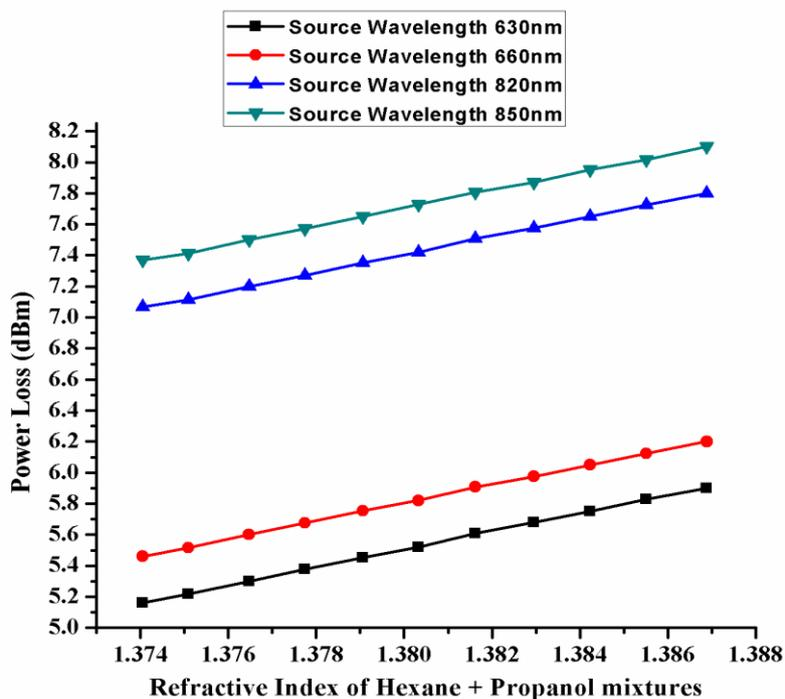
**Fig.6: Relation between Refractive Index of Hexane + Propanol mixtures Vs Power Loss(dBm) for wavelengths of 620nm, 660nm, 820nm & 850nm**
