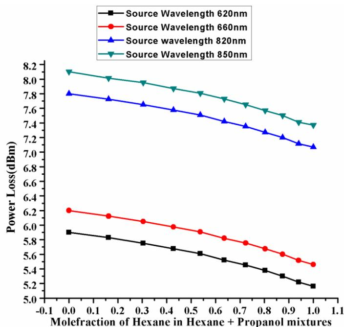
Fig.9: Relation between Molefraction of Hexane in Hexane + Propanol mixtures Vs Power Loss(dBm) for wavelengths of 620nm, 660nm, 820nm & 850nm
