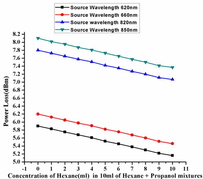
Fig.7: Relation between Concentraion of Hexane(ml) in 10ml of Hexane + Propanol mixtures Vs Output Power(dBm) for wavelengths of 620nm, 660nm, 820nm & 850nm
