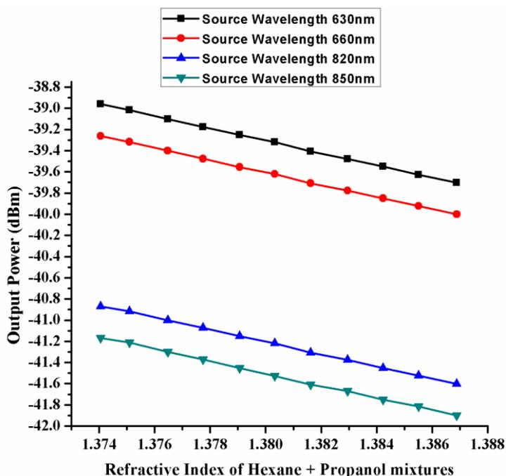
Fig.5: Relation between Refractive Index of Hexane + Propanol mixtures Vs Output Power(dBm) for wavelengths of 620nm, 660nm, 820nm & 850nm
