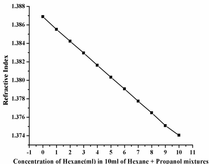
**Fig.3: Relation between Concentration of Hexane(ml) in 10ml of Hexane + Propanol mixtures Vs Refractive Index**
