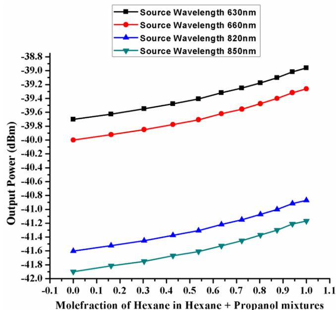
Fig.8: Relation between Molefraction of Hexane in Hexane + Propanol mixtures Vs Output Power(dBm) for wavelengths of 620nm, 660nm, 820nm & 850nm
