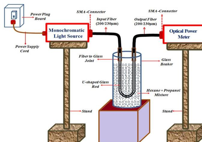
**Fig.1: Experimental Arrangement of Multimode Step-Index Extrinsic Fiber Optic Sensor**
