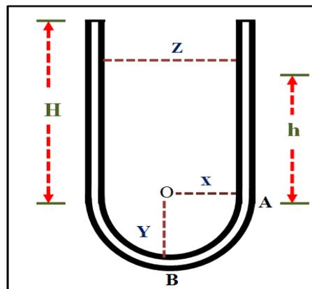
**Fig.2: Geometrical parameters of the U-shaped glass rod**
