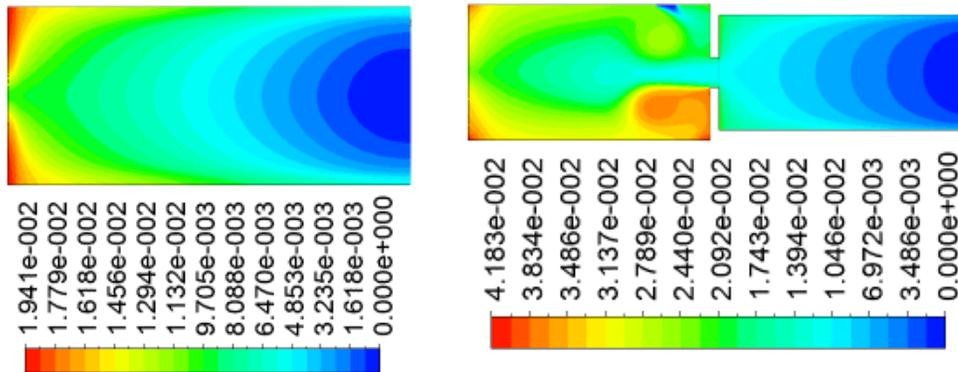
Fig. 14 CO emissions from CCE with gasoline for Set-B and Set-C
