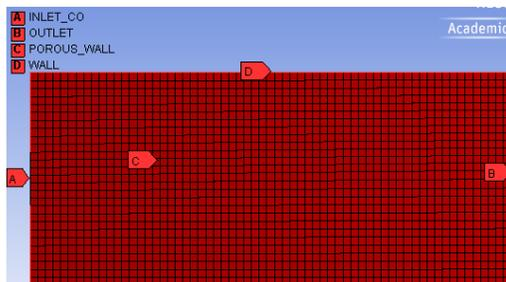
Fig.4 Mesh model with boundary names without air box
