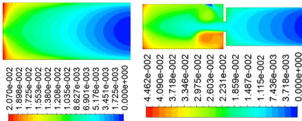
Fig. 15 UBHC emissions from CCE with gasoline for Set-B and Set-C
