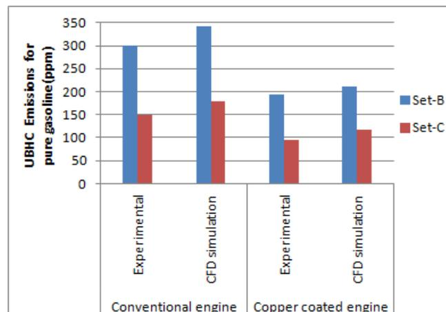
Fig.15 UBHC emissions from experimental and CFD for Set-B & Set-C with both versions of engine using pure gasoline
