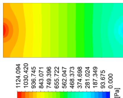
Fig.8 Back pressure in catalytic converter without air box
