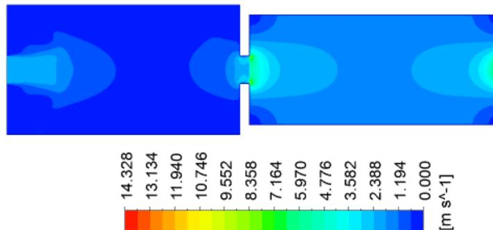
Fig.7 Flow of velocity in air box and catalytic converter
