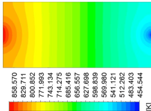
Fig.10 Temperature flow in catalytic converter without air box
