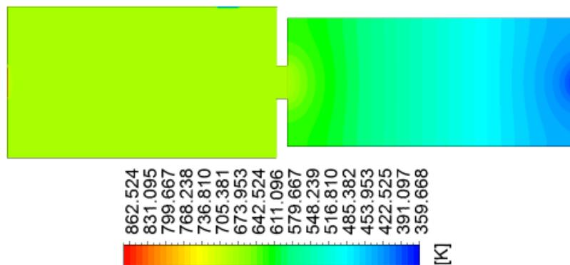
Fig.11 Temperature flow in catalytic converter with air box
