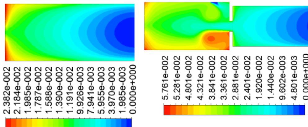
Fig. 12 CO emissions from CE with pure gasoline for Set-B and Set-C
