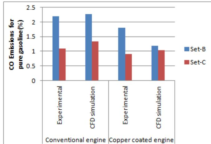
Fig.14 CO emissions from experimental and CFD for Set-B & Set-C with both versions of engine using pure gasoline
