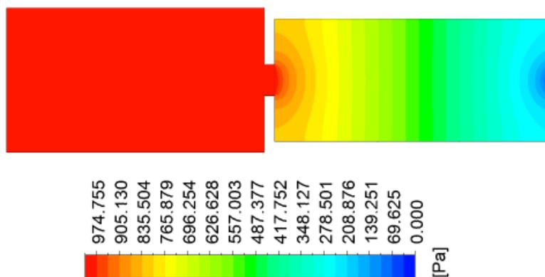
Fig.9 Back pressure in catalytic converter with air box
