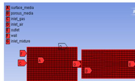
Fig.5 Mesh model boundary names with air box
