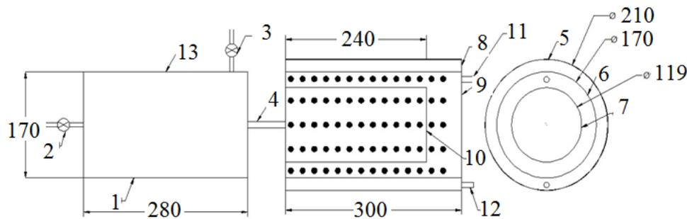
Fig. 1 Details of catalytic converter. (All dimensions are in mm)
