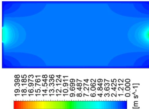
Fig.6 Flow of velocity in catalytic Converter
