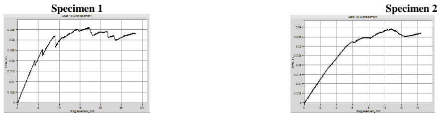
Fig 4 Load v/s displacement Graph of Specimen 1 & 2 with fiber: resin volume fraction of 30:70
