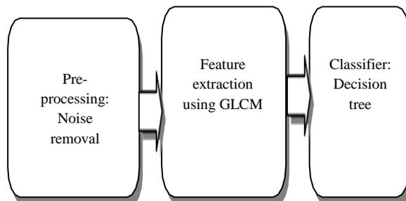
Fig.3(b) Block diagram for Decision Tree algorithm
