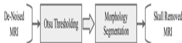
Fig.1Process flow of skull stripping using mathematicalmorphology
