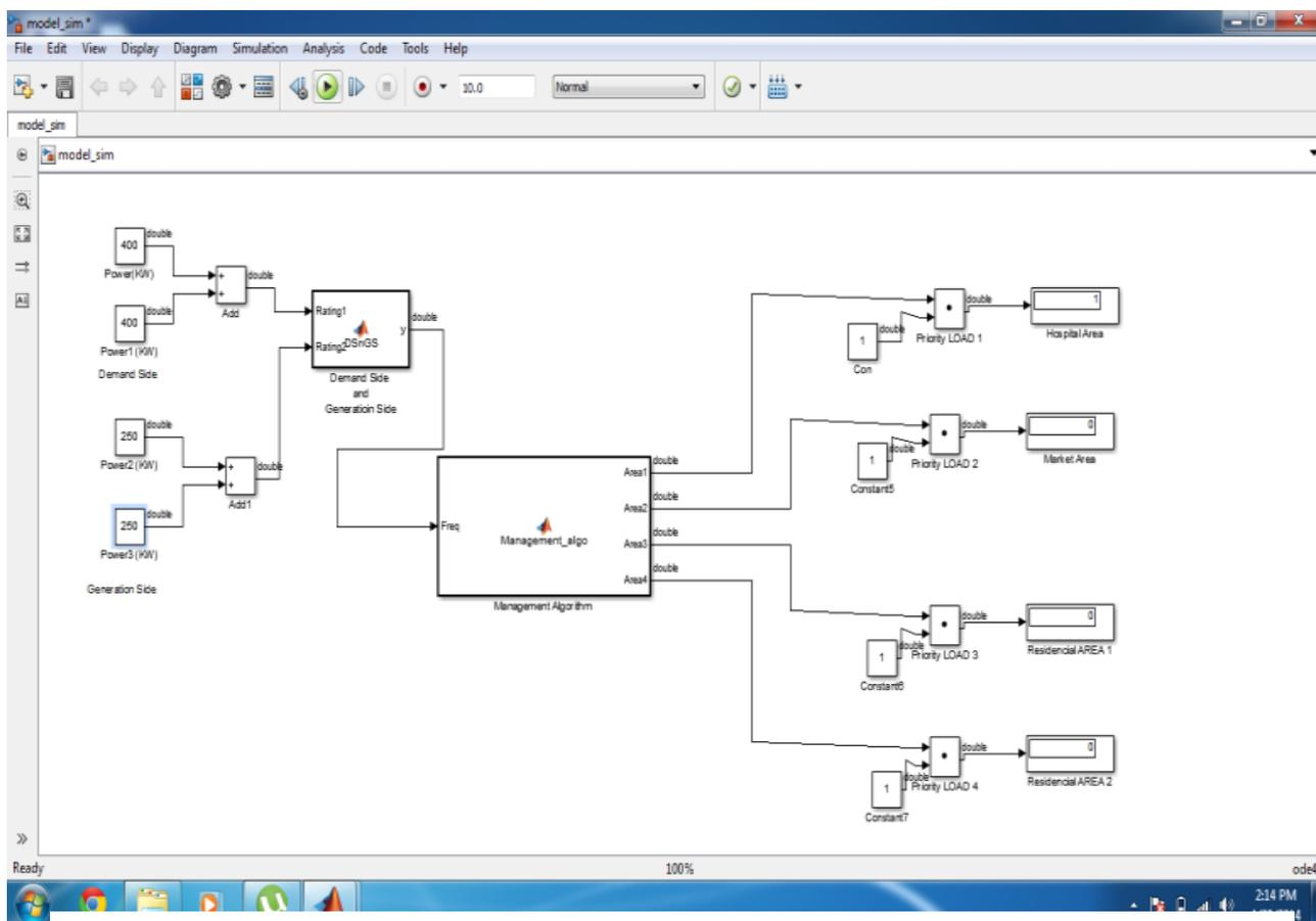
In Figure 4.2, adder at demand side collects 800kW power, while the Generation side adder collects 500kW. At this time, Demand is greater than that of generation side. So it affected the frequency and frequency is fallen down to 49.5Hz, as a result the loads except restricted areas are shed.
