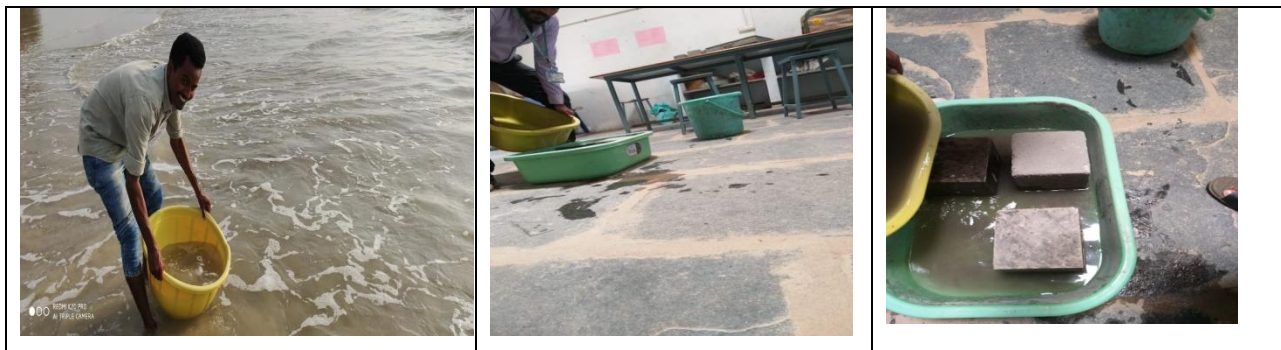
Fig 1: Sea water sample collection and immersion of cubes in the sea water
