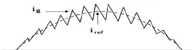
Fig. 3. Waveforms of reference current and inductor current
