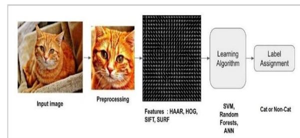
Fig.3. Working of Image Recognition.
