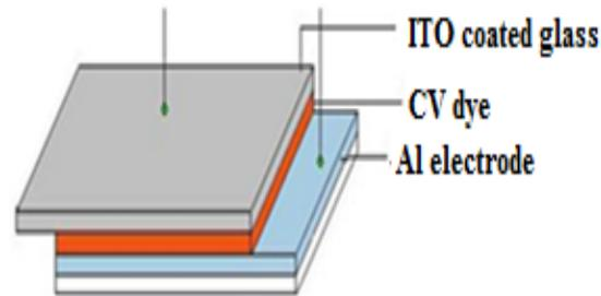
Fig. 2 Schematic diagram of the organic device
