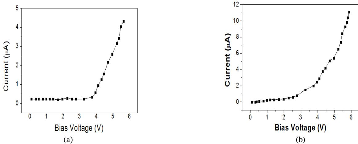
**Fig.3 Dark I-V characteristics of organic device comprising of CV dye (a) without SWCNT and (b) with SWCNT**
