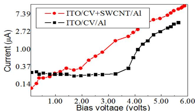
Fig.4 In I-V characteristics of CV dye based device with and without SWCNT
